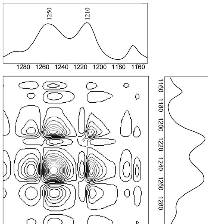
FIG. 8. Synchronous 2D-IR of the PO-PPV precursor in the ether stretch region, 1300–1150  $\text{cm}^{-1}$ .
