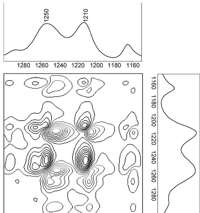
FIG. 9. Asynchronous 2D-IR of the PO-PPV precursor in the ether stretch region, 1300–1150  $\text{cm}^{-1}$ .
