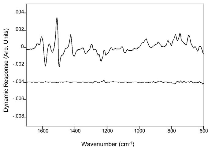
FIG. 4. (Top) Dynamic in-phase and (bottom) quadrature spectra (1650–600  $\text{cm}^{-1}$ ) of PO-PPV offset on the same scale.
