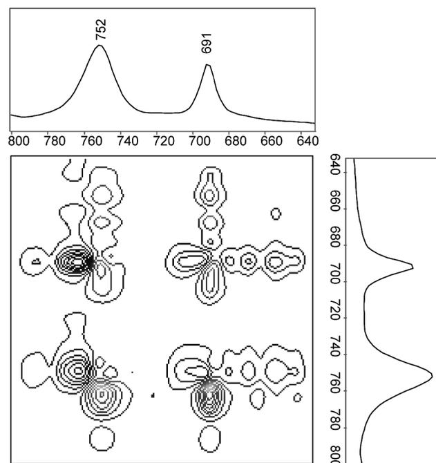
FIG. 11. Asynchronous 2D-IR of the PO-PPV precursor in the phenoxy C–H out-of-plane bend region, 800–600  $\text{cm}^{-1}$ .
