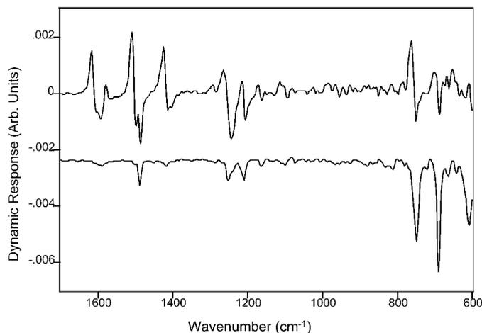
FIG. 3. (Top) Dynamic in-phase and (bottom) quadrature spectra (1650–600  $\text{cm}^{-1}$ ) of the PO-PPV precursor offset on the same scale.
