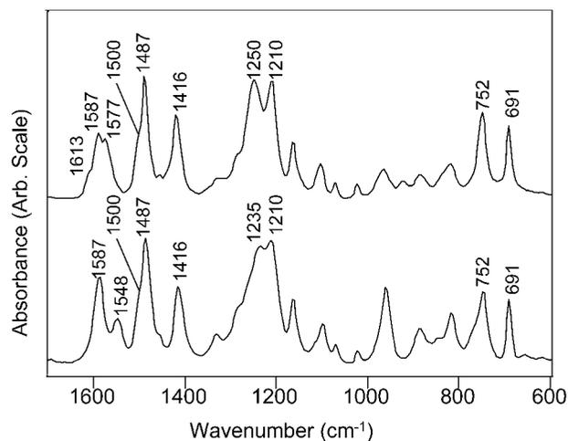
FIG. 2. Infrared absorbance spectra (1650–600  $\text{cm}^{-1}$ ) of (top) the PO-PPV precursor and (bottom) PO-PPV obtained in rapid-scan mode.
