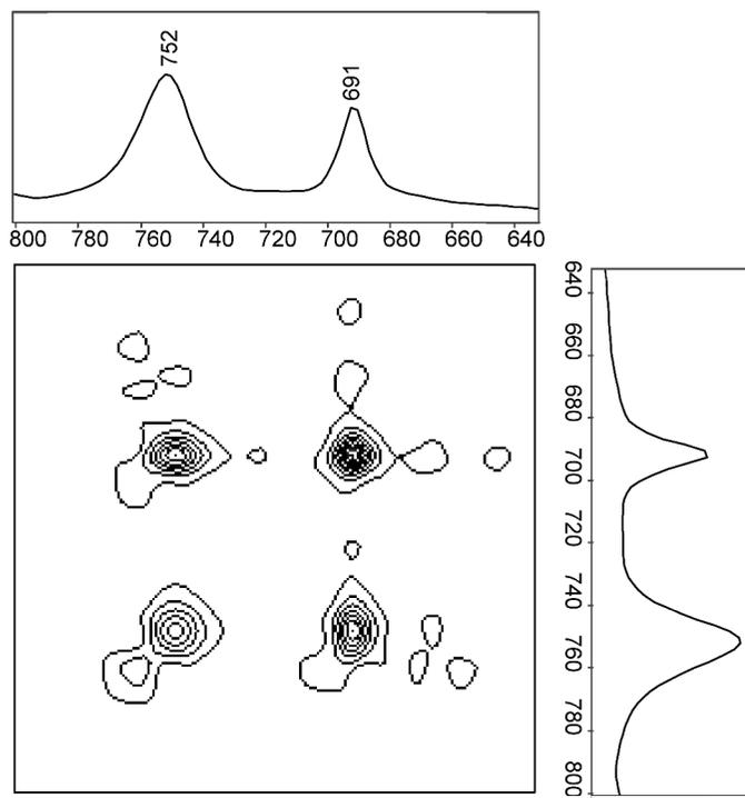
FIG. 10. Synchronous 2D-IR of the PO-PPV precursor in the phenoxy C–H out-of-plane bend region, 800–600  $\text{cm}^{-1}$ .
