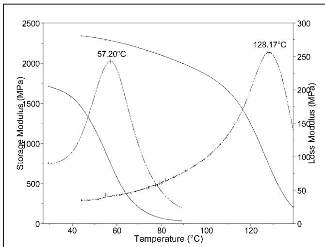
FIG. 12. The storage (solid) and loss (dashed) modulus of PO-PPV (both right) and the PO-PPV precursor (both left) over the temperature range 25–140 °C.
