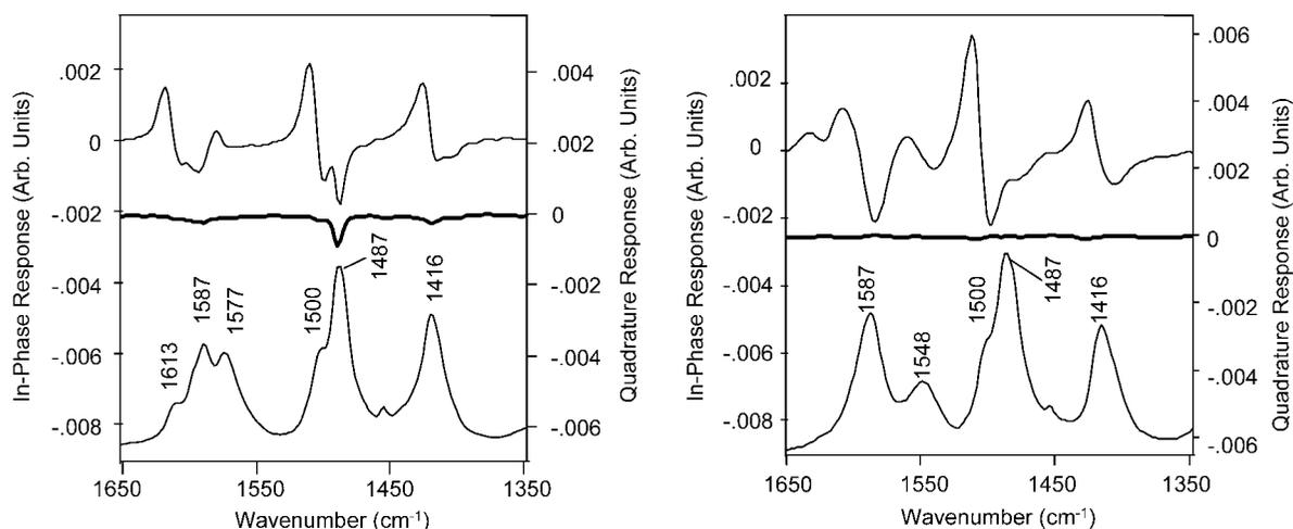
FIG. 5. (Left) Dynamic (in-phase (top) and quadrature (middle, bold)) and absorbance spectra (bottom) (with peak labels) of the PO-PPV precursor in the ring stretch region, 1650–1350  $\text{cm}^{-1}$ . (Right) Dynamic (in-phase (top) and quadrature (middle, bold)) and absorbance spectra (bottom) (with peak labels) of PO-PPV in the ring stretch region, 1650–1350  $\text{cm}^{-1}$ .
