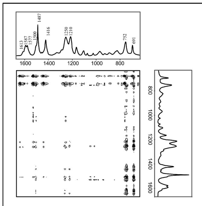
FIG. 7. Asynchronous 2D-IR of the PO-PPV precursor in the 1650–600  $\text{cm}^{-1}$  region.
